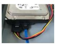
**⑤**Connect the HDD cable and power cable.
