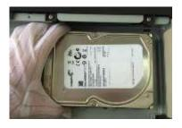
③ Place the HDD in accordance with the four holes in the bottom.
